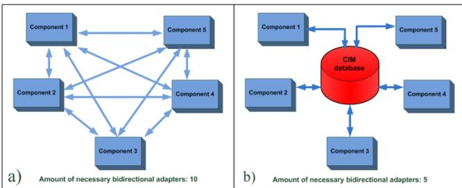
Fig. 6. Amount of necessary data conversions between several SW-components a) without and b) with CIM. Each arrow represents a bidirectional adapter.
