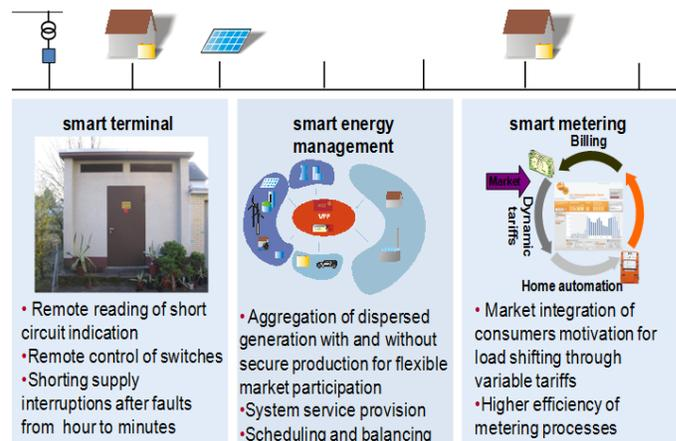
Fig. 1. Pillars of a smart distribution network
