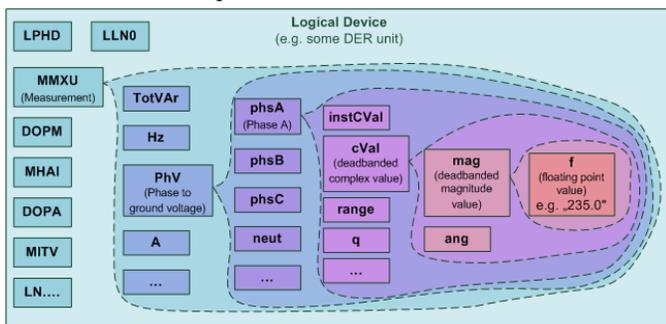
Fig. 4. Example of assigning a given measured value to the designated space in IEC 61850 communication protocol: The measured value of 235.0 V of phase A is assigned to the float field, contained inside the class hierarchy of the logical node MMXU.
