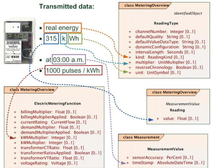
Fig. 7. Mapping of meter data to the appropriate CIM classes
