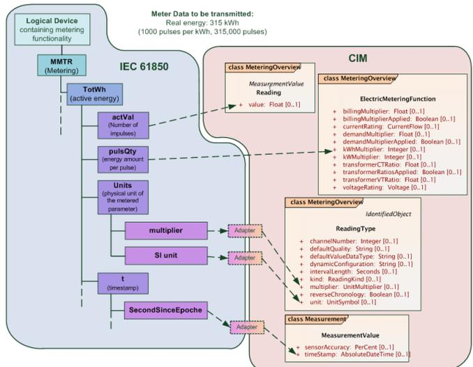
Fig. 8. Mapping of data communicated in IEC 61850 to CIM database scheme
