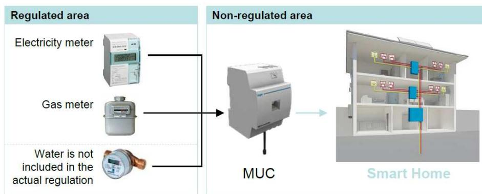
Fig. 2: Concept of modules (meter and communication controller)
